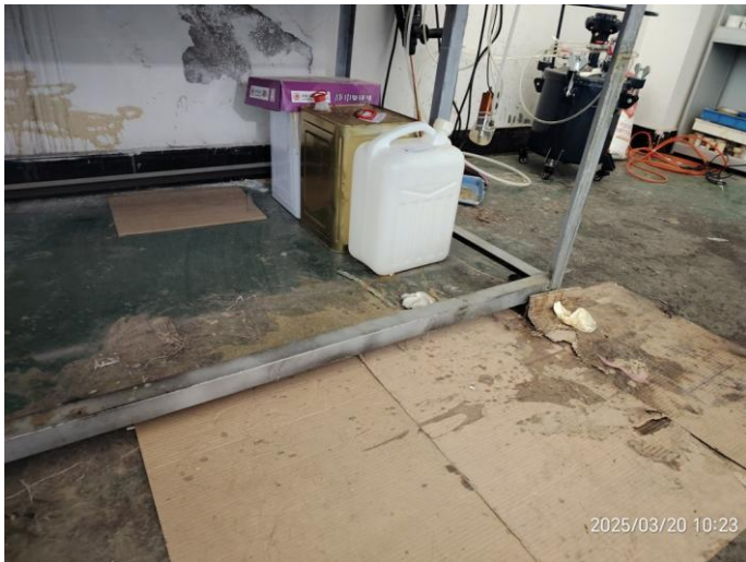
NC 7.7 Chemical missing secondary containment
